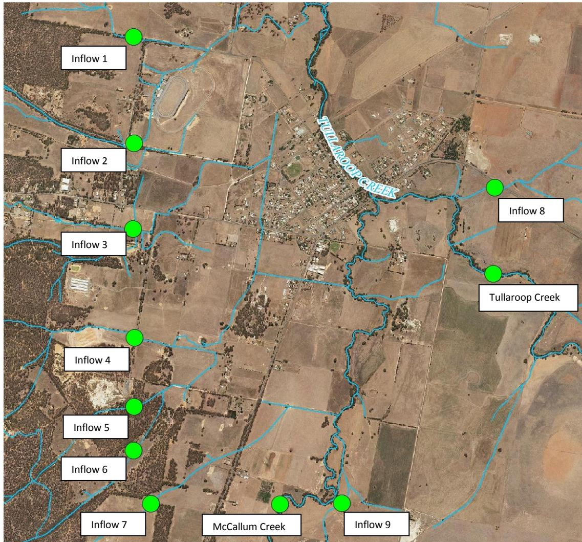
**Figure 4-3** Location of RORB extracted hydrographs around Carisbrook
