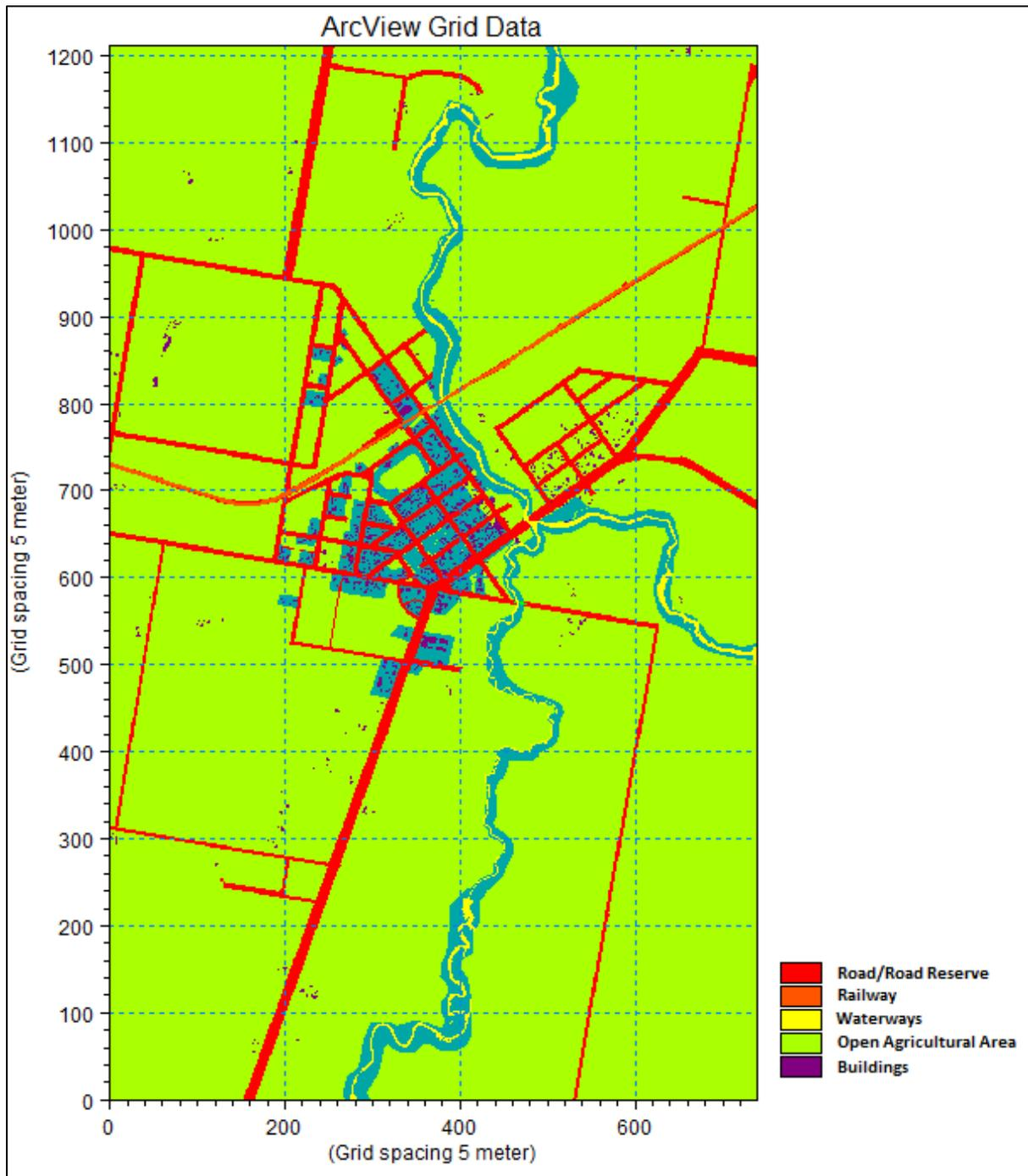
Figure 5-2 2D hydraulic model roughness grid
