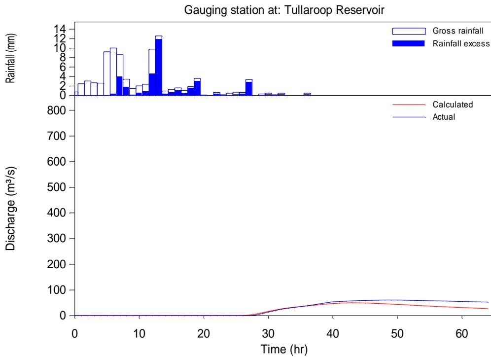
**Figure 4-19 RORB model calibration hydrograph – September 2010 at Tullaroop Head Gauge**
