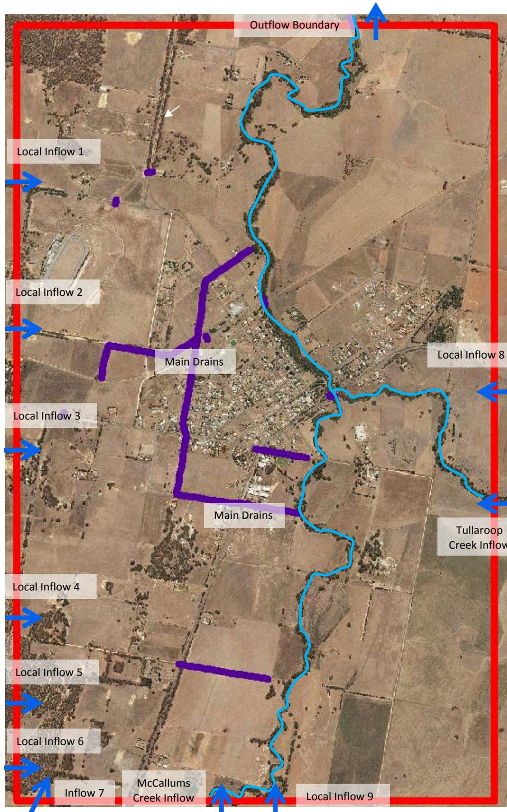
Figure 5-3 Conceptual hydraulic model extents and boundary locations
