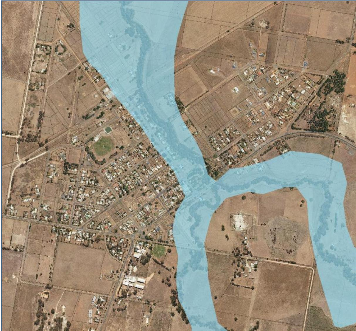
**Figure 1-2 Existing Land Subject to Inundation Overlay for Carisbrook (VFD)**
