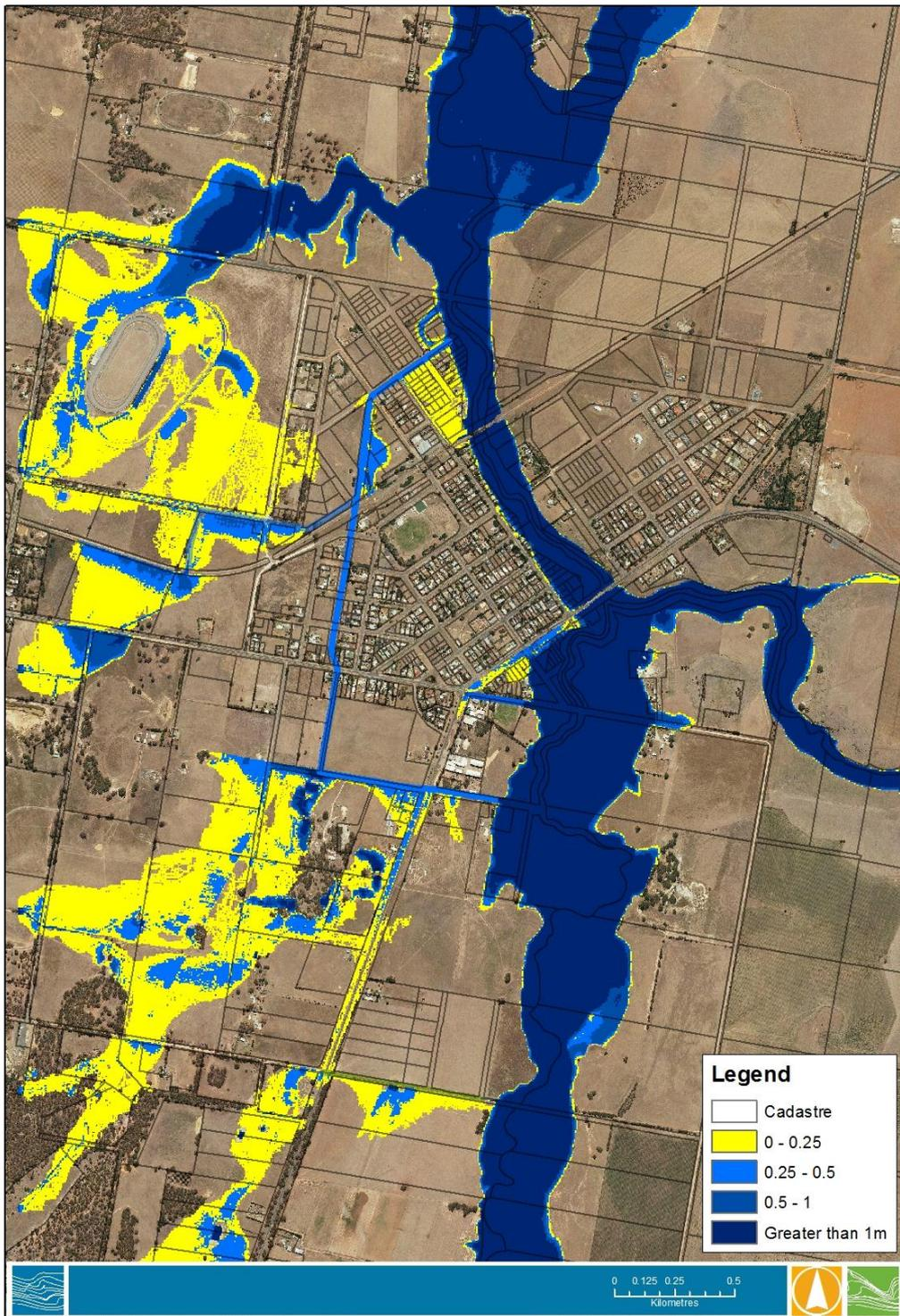
**Figure 6-7 Mitigation Option 2 (highway alignment) – 100 year ARI depth results**
