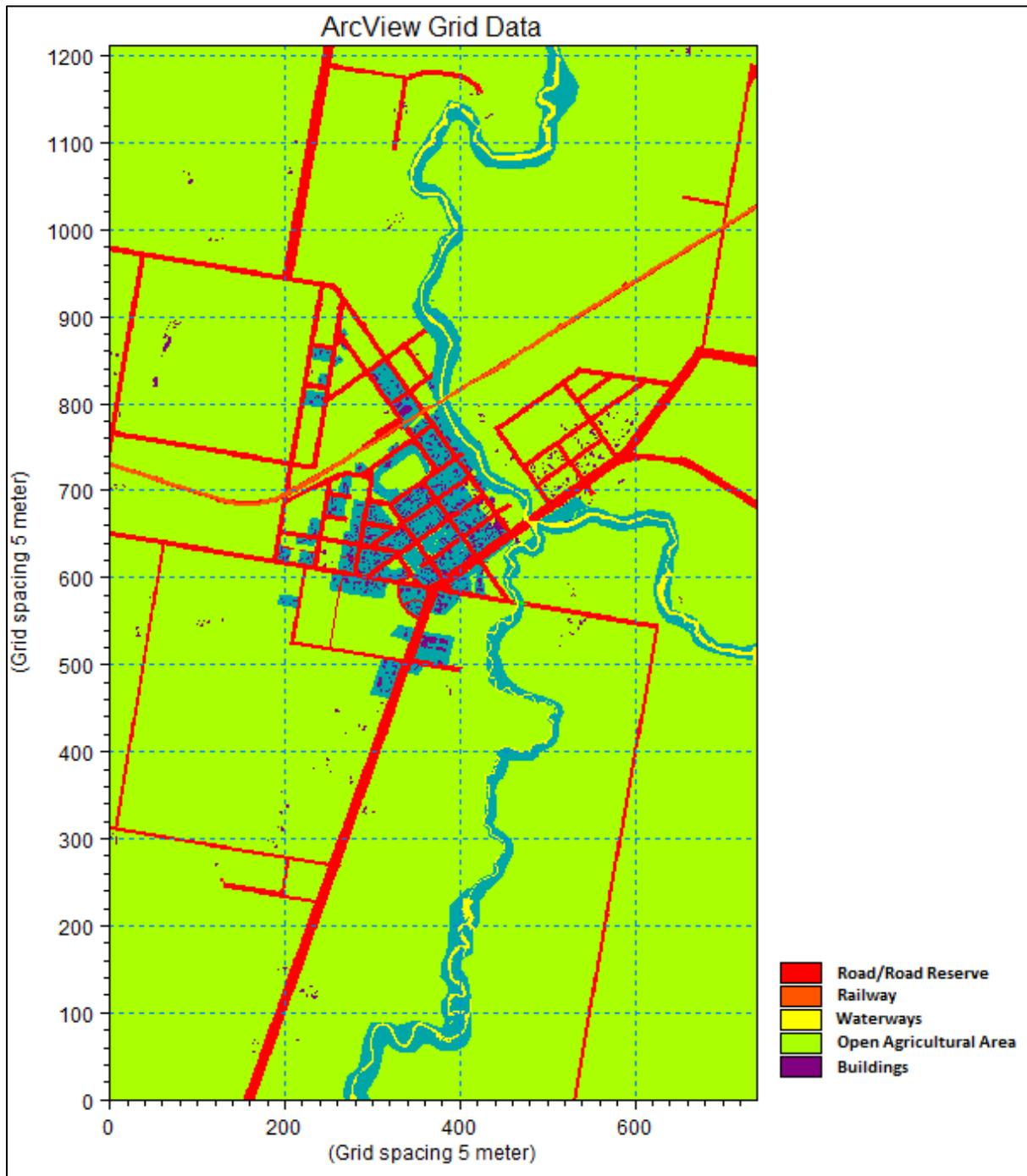
Figure 5-2 2D hydraulic model roughness grid
