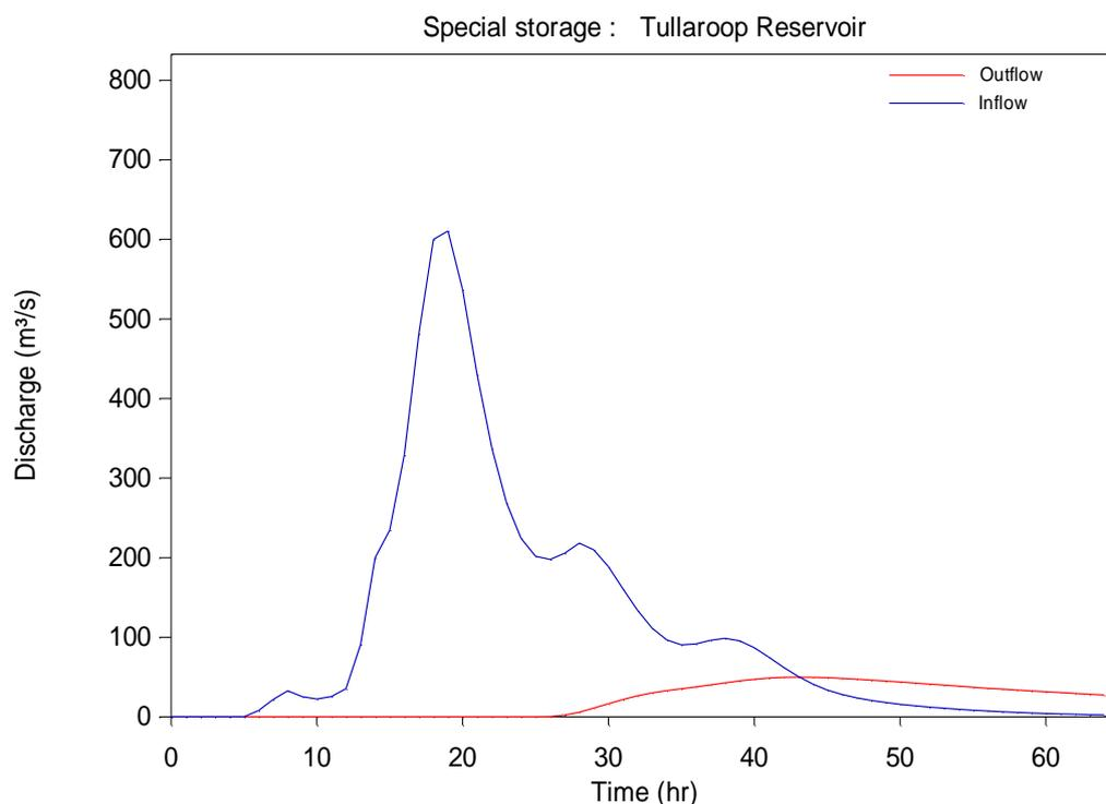
**Figure 4-21 RORB model calibration hydrograph – Inflow/Outflows at Tullaroop Reservoir during September 2010 event**
