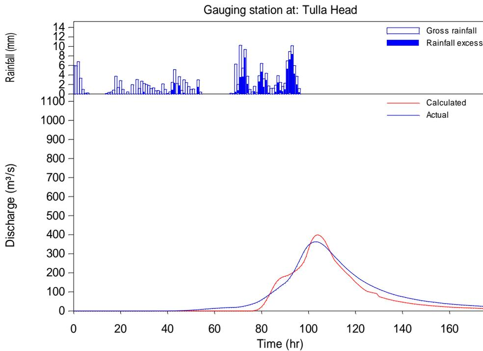
**Figure 4-15 RORB model calibration hydrograph – January 2011 at Tullaroop Head Gauge**
