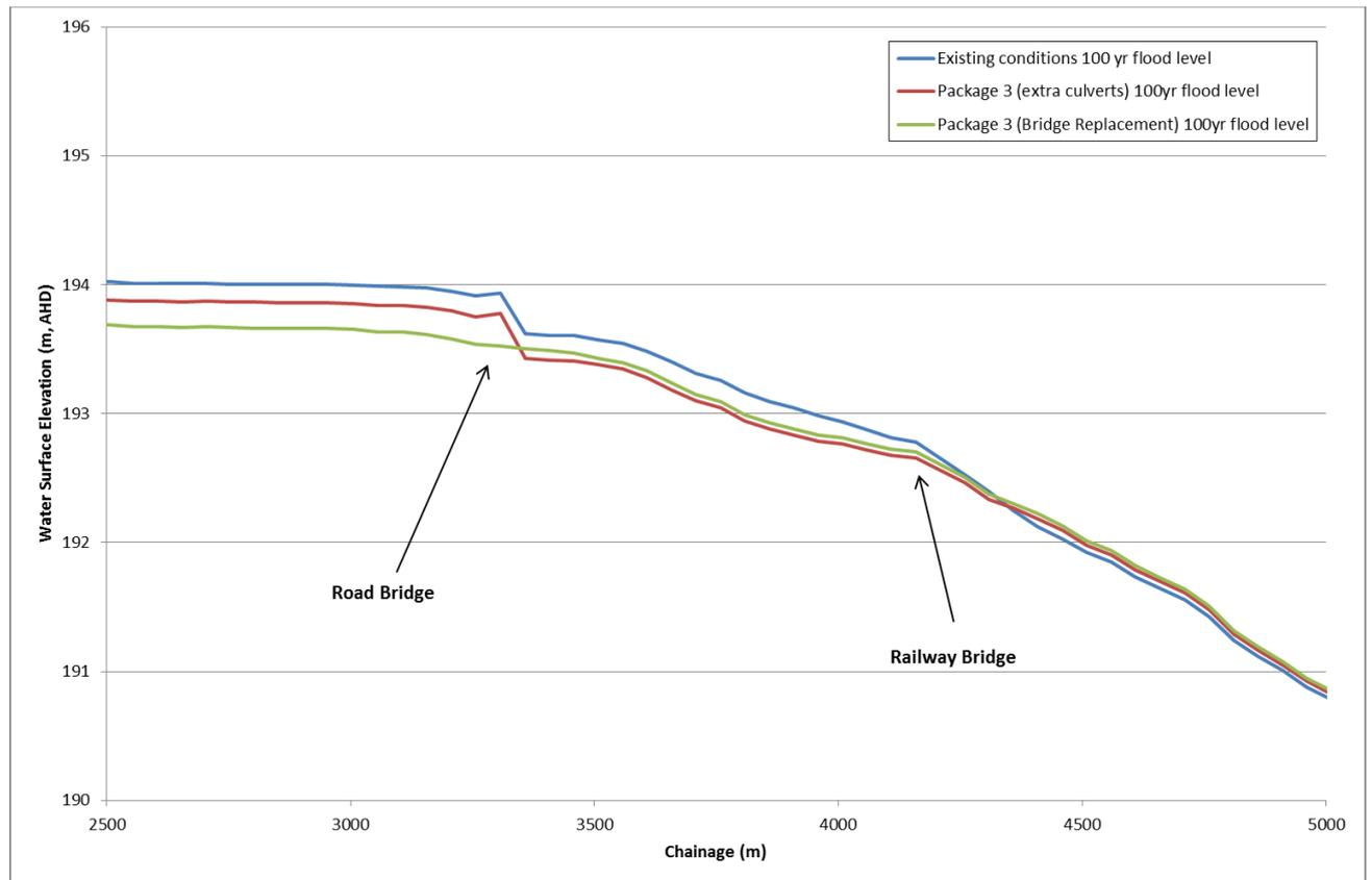
**Figure 6-9 Long-section plot of Package 3 results**
