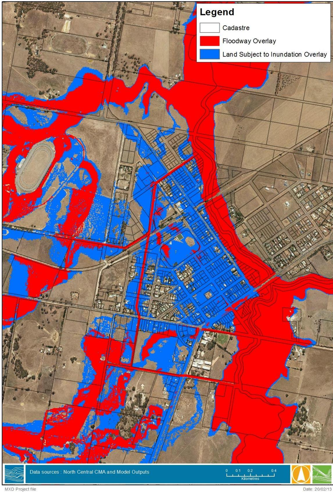
**Figure 6-16** Draft LSIO and FO Map for Existing Conditions
