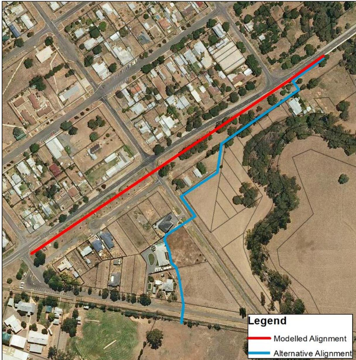
Figure 6-6 Option 2 Modelled and Alternative Levee Alignments
