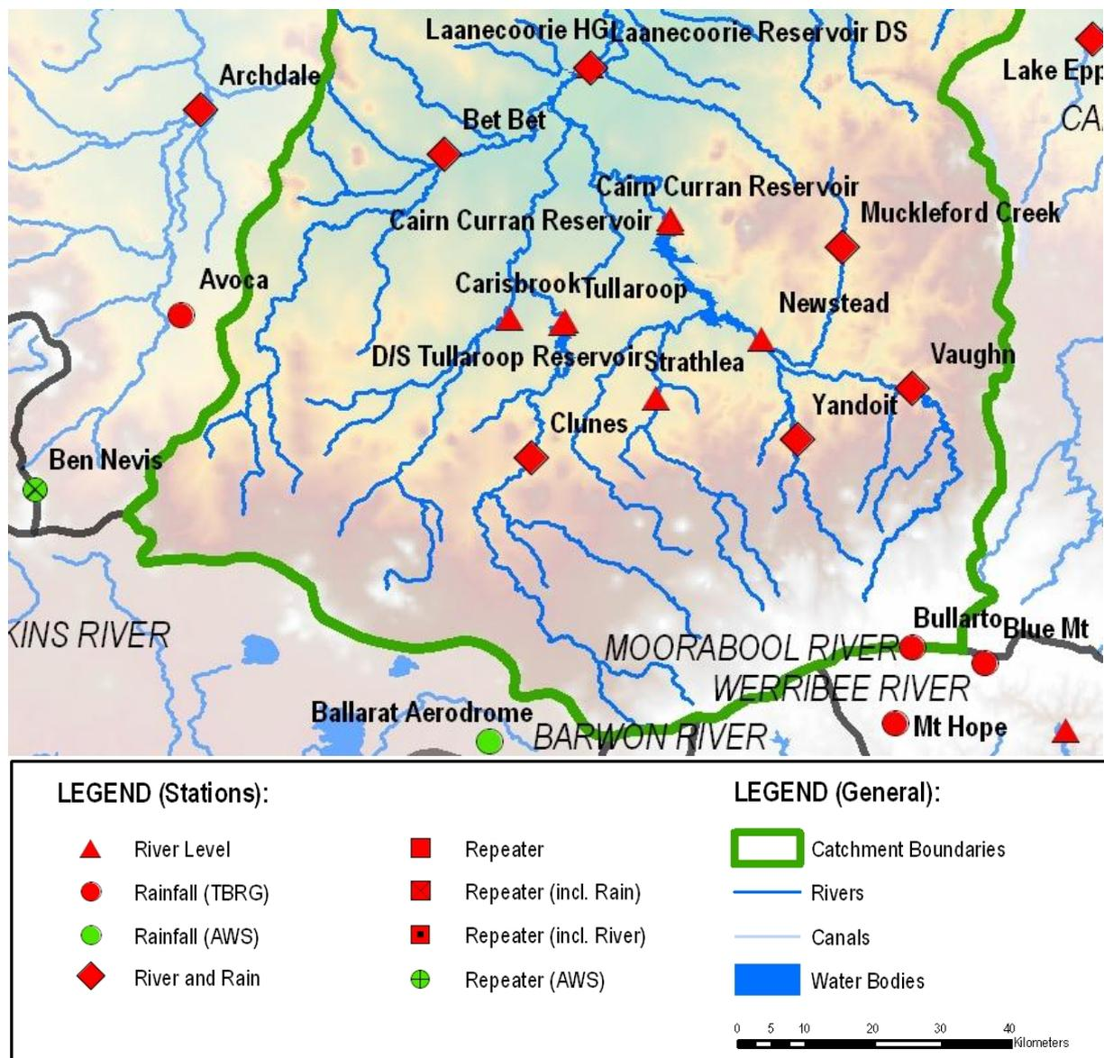
**Figure 2-1 Existing flood warning data collection network in the vicinity of Carisbrook**
