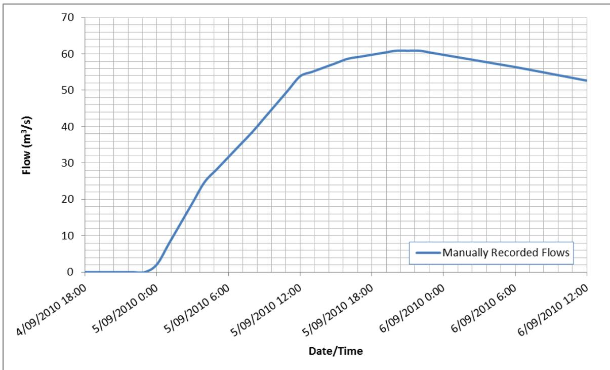
**Figure 4-5 Tullaroop Creek @ Tullaroop Reservoir flow hydrograph – September 2010**
