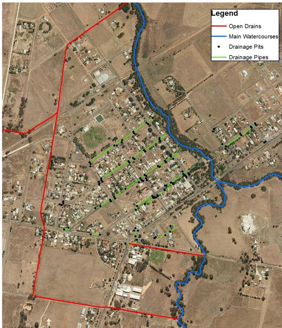
Figure 3-6 Carisbrook Drainage Network (Central Goldfield Shire)
