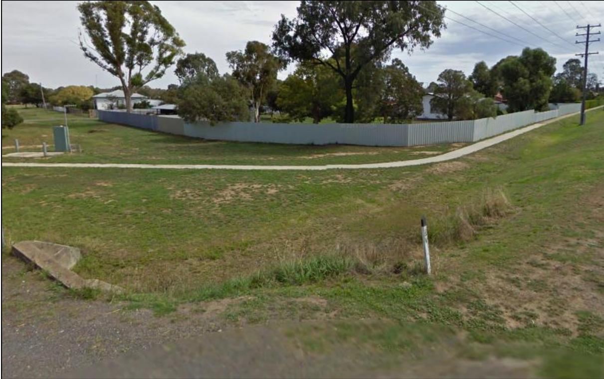
**Figure 3-7** Typical swale drain at corner of Pyrenees Highway and Landrigan Road
