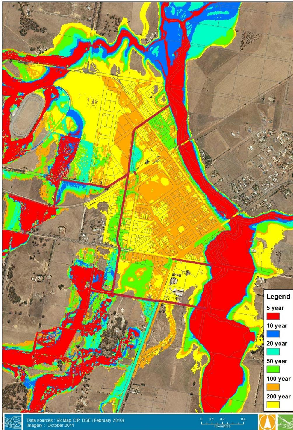
Figure 5-10 Hydraulic modelling design flood extents
