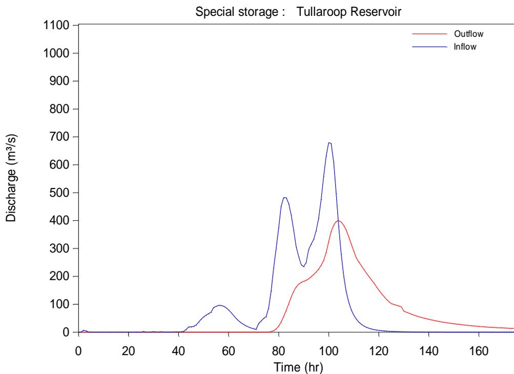
**Figure 4-18 RORB model calibration hydrograph – Inflow/Outflows at Tullaroop Reservoir during January 2011 event**
