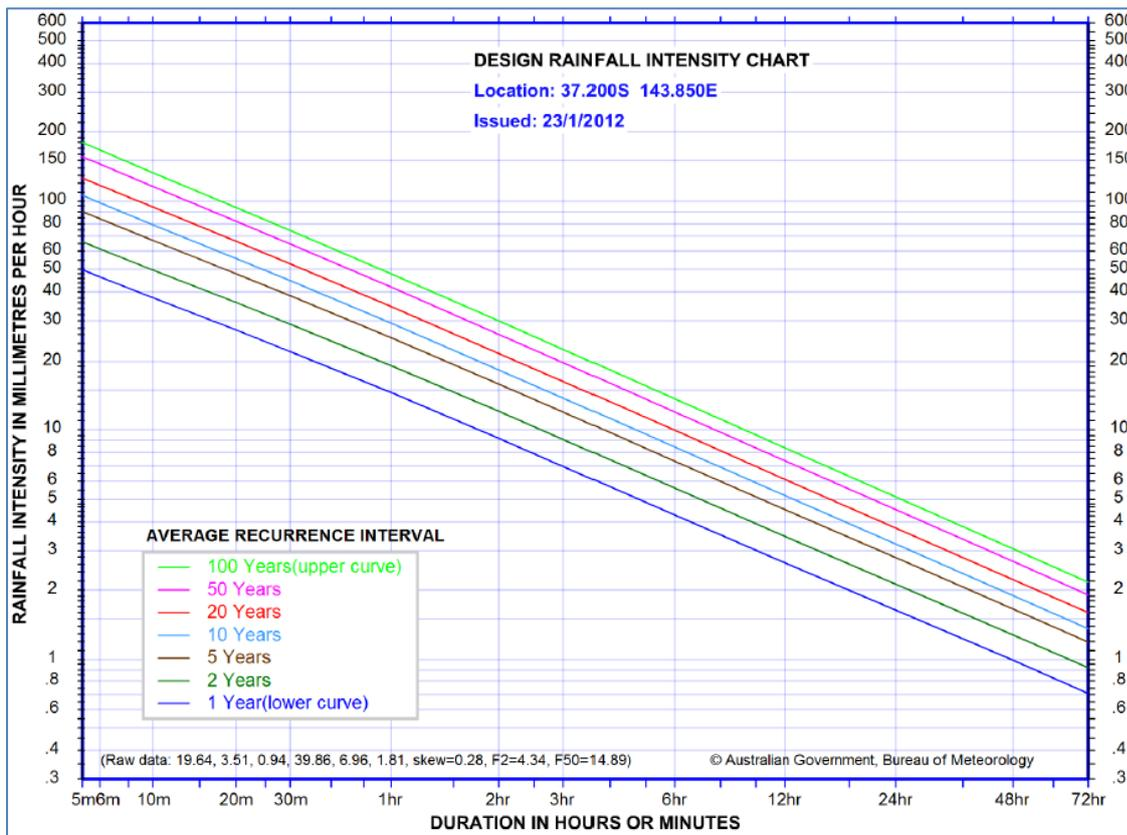
**Figure 4-24 IFD curves extracted from the BoM online IFD tool for Carisbrook Catchment**
