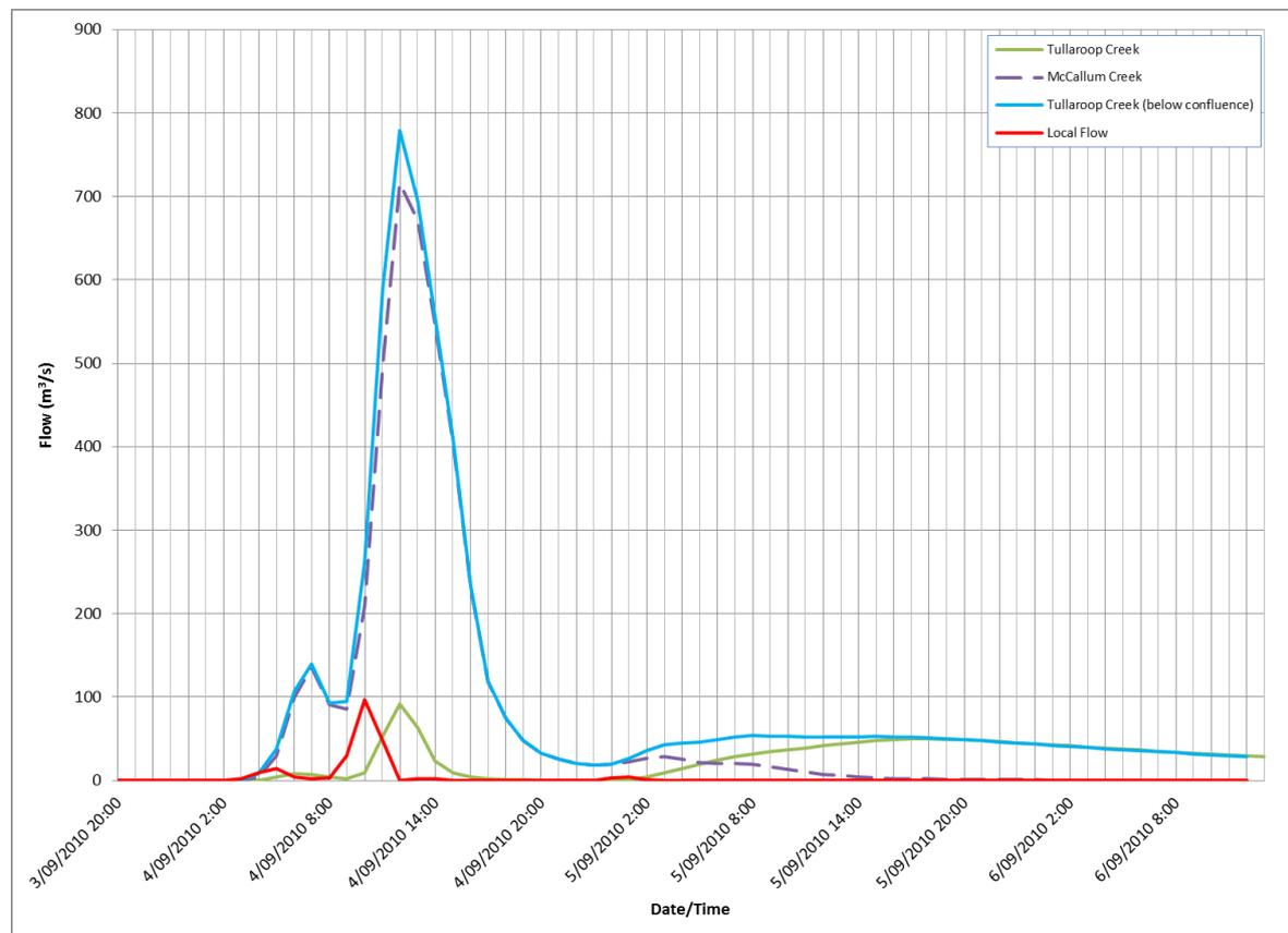
**Figure 4-22 Flood hydrographs in Carisbrook – September 2010**
