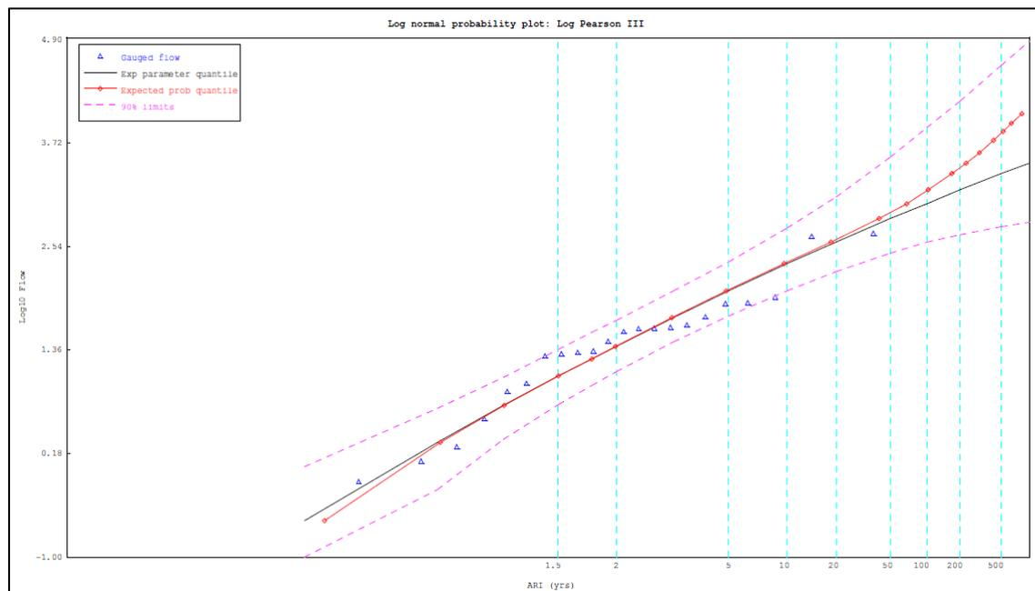
**Figure 4-27 Log Pearson III flood frequency analysis – Tullaroop Reservoir Head Gauge**
