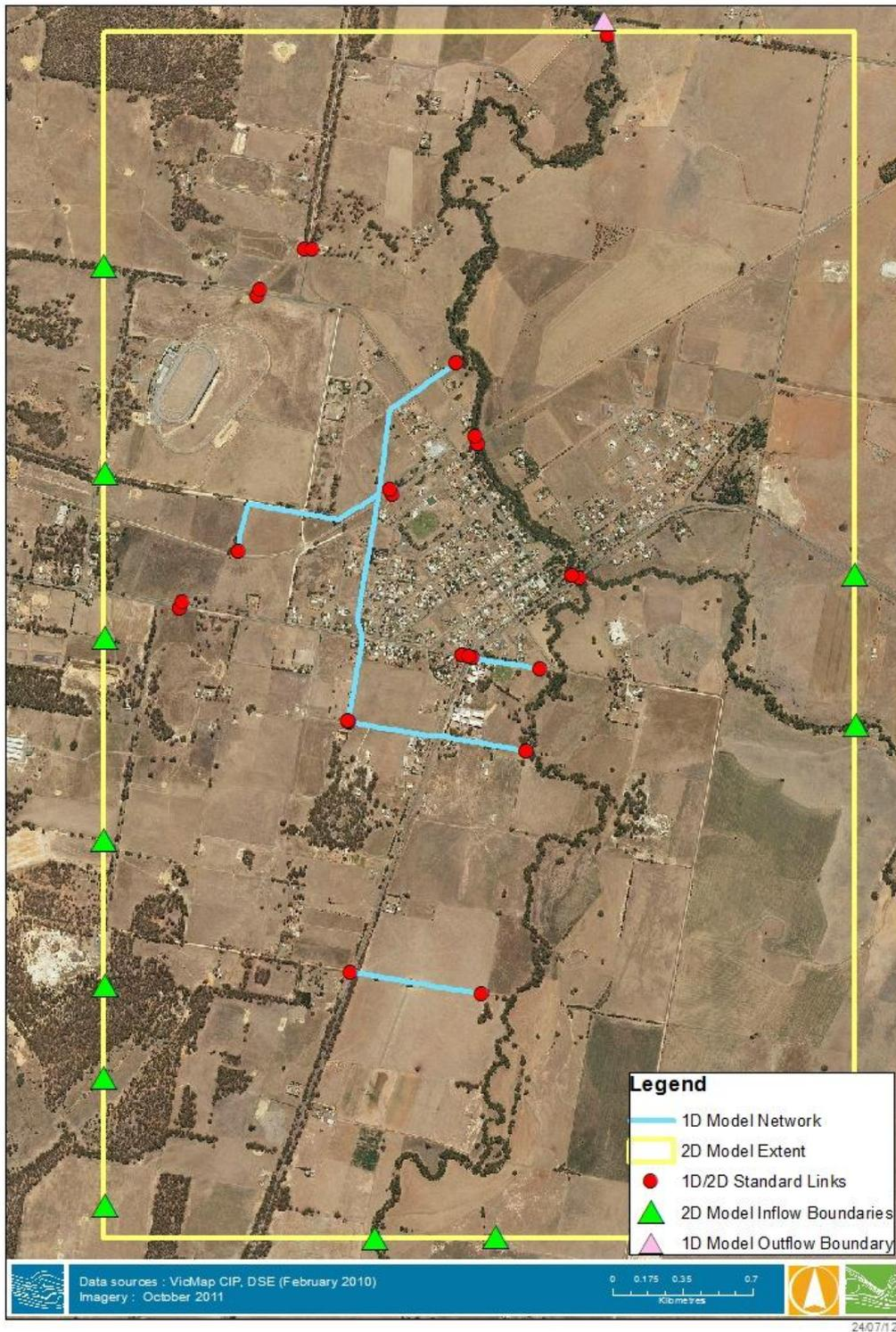
Figure 5-1 1D/2D Hydraulic Model Schematization
