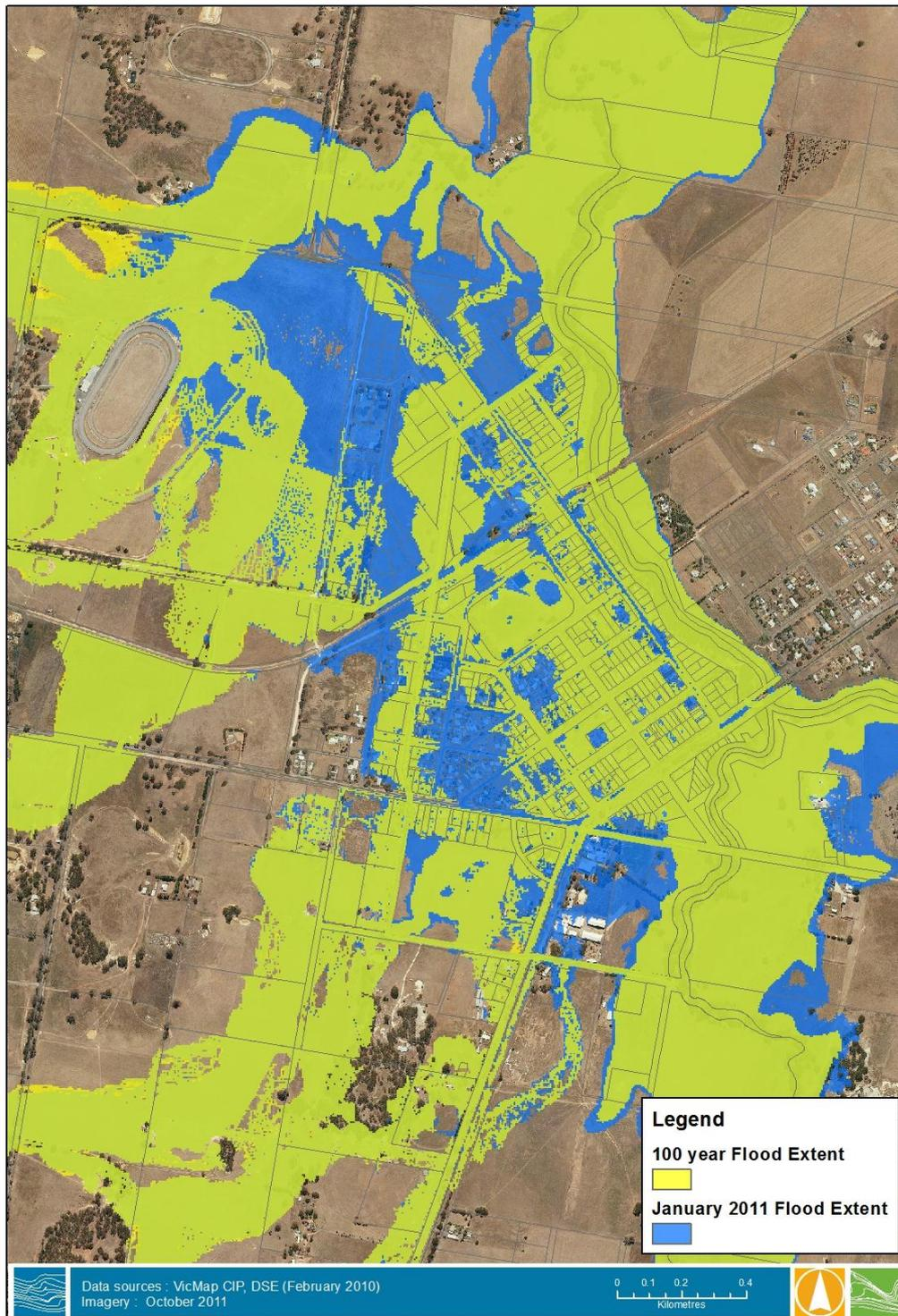
Figure 5-9 Hydraulic Modelling January 2011 and 100 Year ARI Design Event Flood Extents
