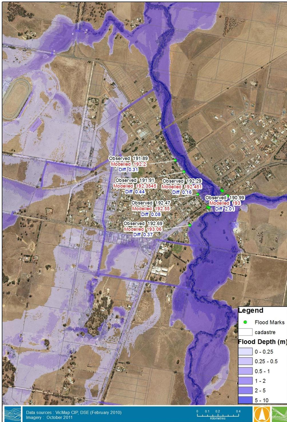
Figure 5-4 Hydraulic model calibration plot – September 2010
