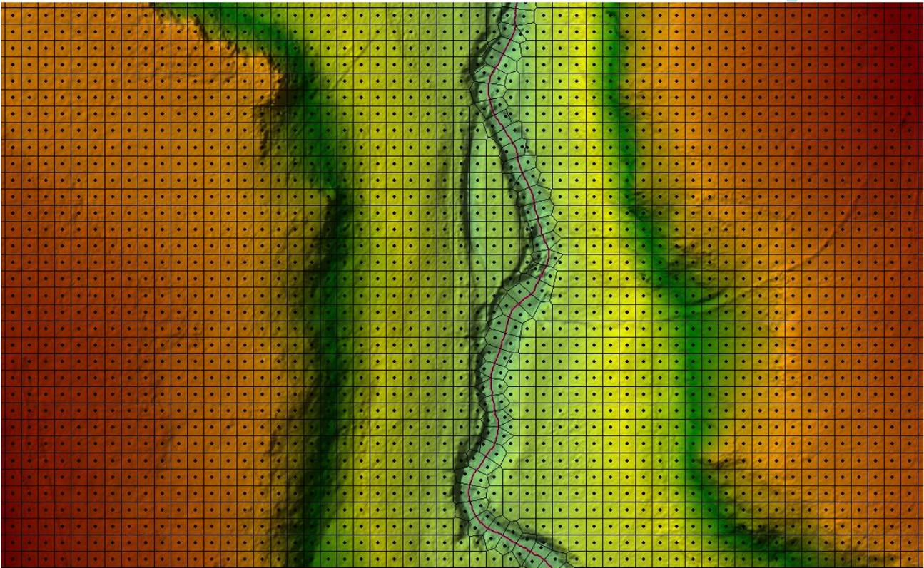
Figure 3 – Example of cell delineation within the hydraulic model
