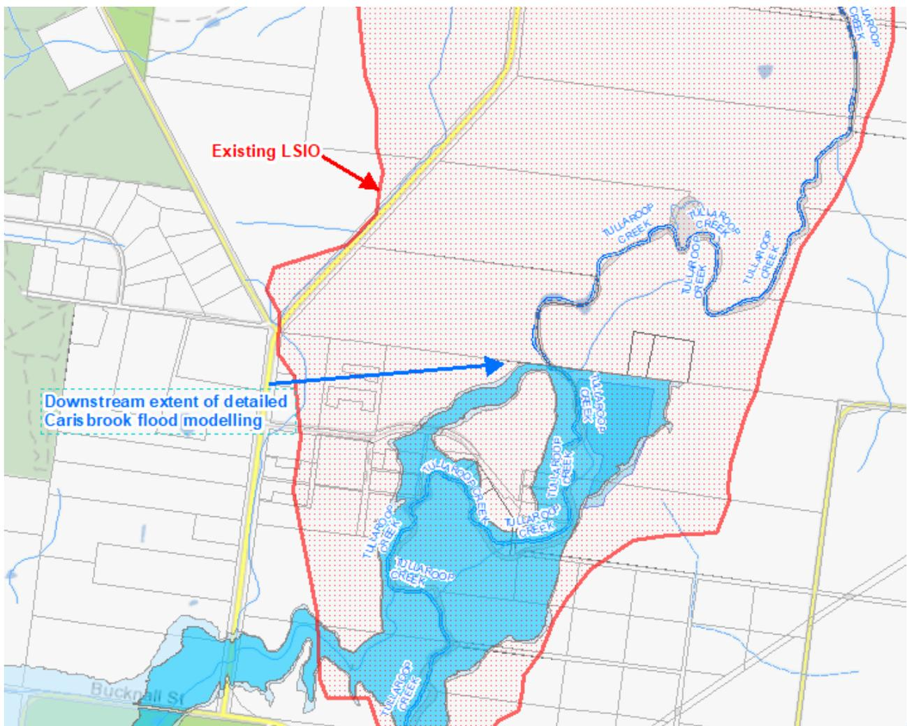
Figure 1 – Interface between existing LSIO and downstream boundary of detailed Carisbrook flood modelling
