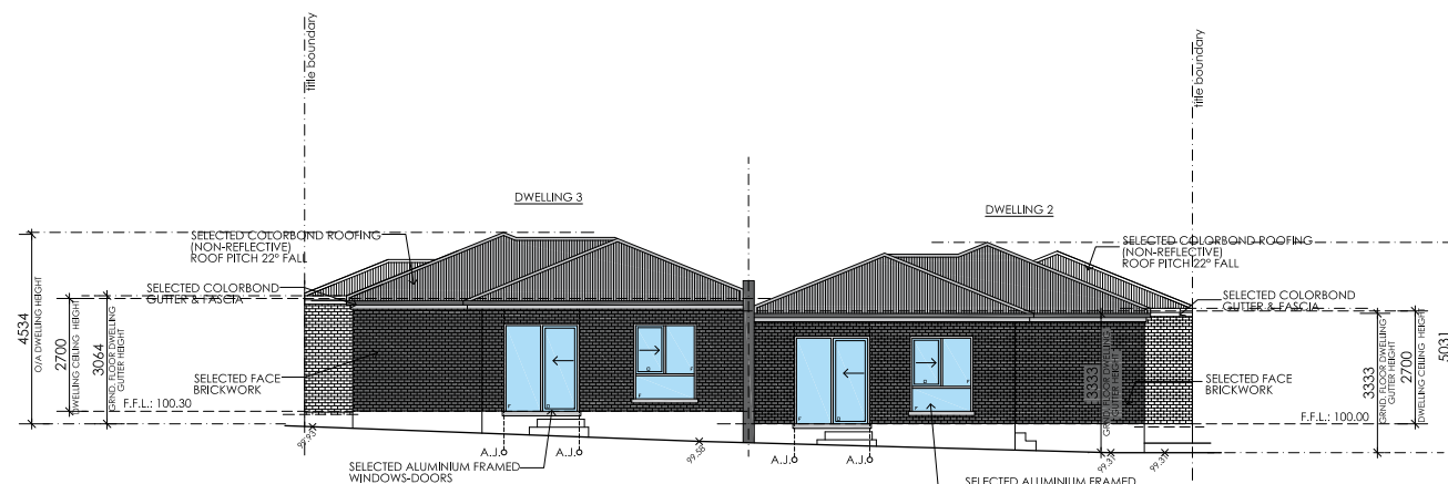
EAST ELEVATION: DW2 & DW3 1:100
